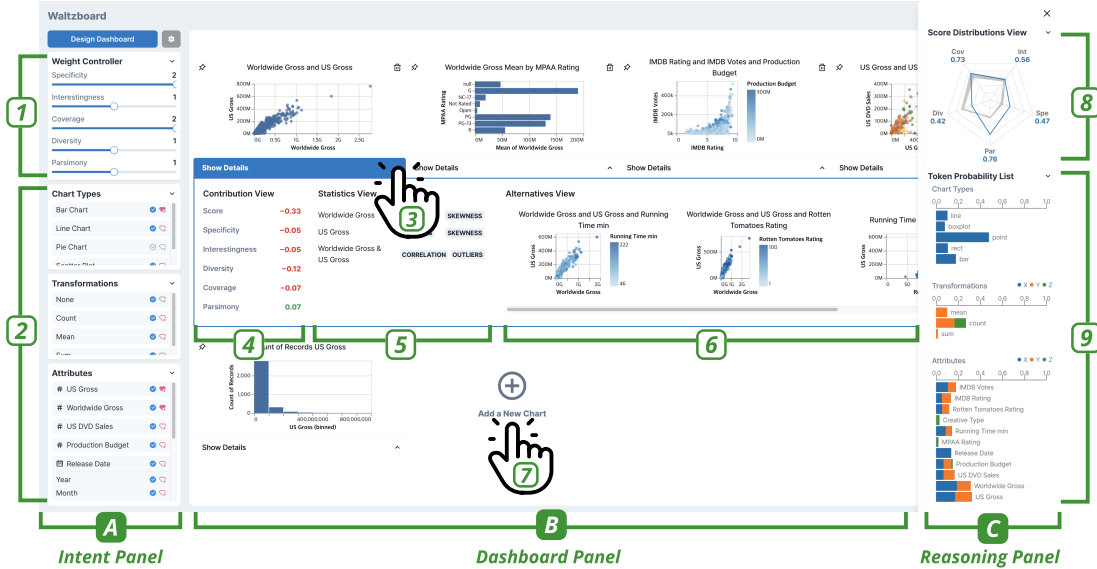
Figure 1: The user interface of Waltzboard . A The Intent Panel allows the user to flexibly express their intent by tuning the weights of five measures (1) and prioritizing chart types of attributes of interest (2). B The Dashboard Panel shows a dashboard generated automatically with the contribution of each chart to the measures (4) and (5) and its alternatives (6). C The Reasoning Panel provides the details of the automatic design process, e.g., the score of the current design compared to alternatives.
